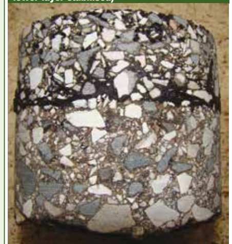
Figure 1 - Experimental results – average values (in the photo, a test piece with its lower layer stabilised)
