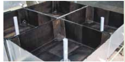
2. Test containers waterproofed with DEFEND ANTIRADICE
