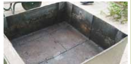
8. Unchanged upper face of DEFEND ANTIRADICE after the testdopo il test
