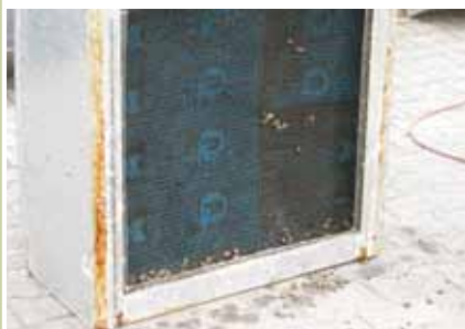
9. Unchanged under face of DEFEND ANTIRADICE after the testdopo il test
