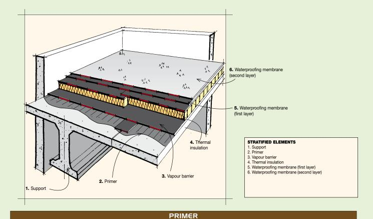
The primer penetrates into the pores of concrete surfaces, stops dust and has the job of promoting adhesion on the surfaces to which the membranes must be stuck. INDEVER is a traditional solvent-based bituminous primer; the ECOVER water-based primer is more innovative
