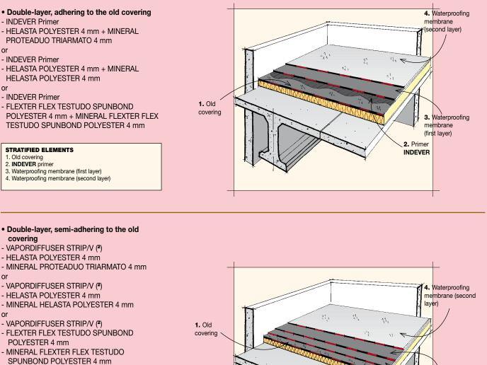
(\*) The use of VAPORDIFFUSER STRIP/V, given the high adhesion level of the adhesive strips distributed on its lower face, means primer does not need to be applied
