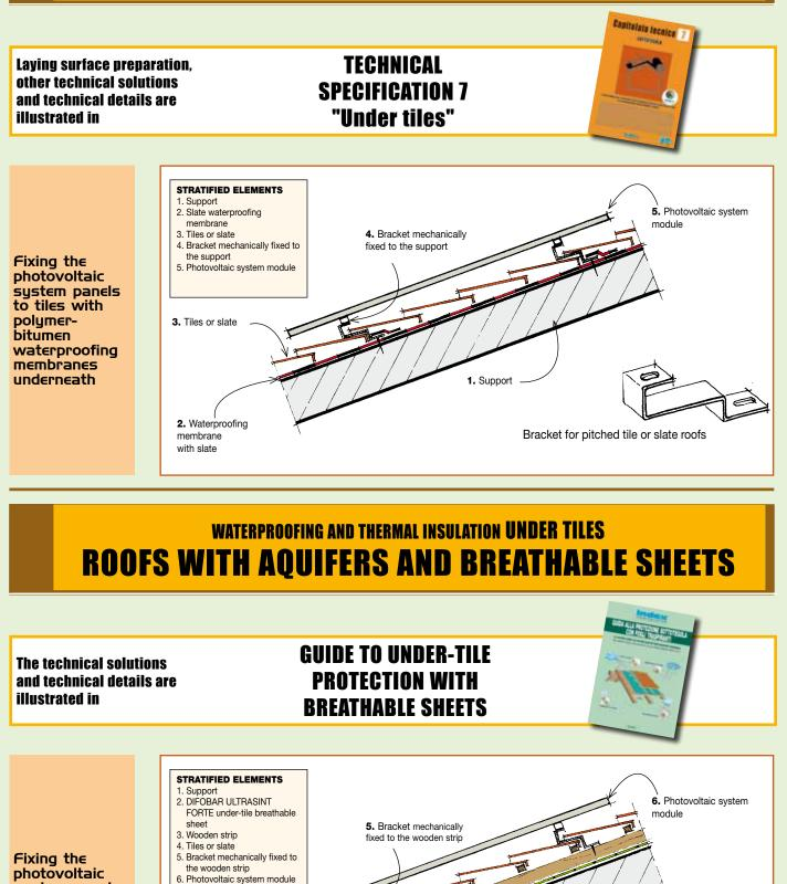
system panels to tiles with breathable sheet protection underneath
